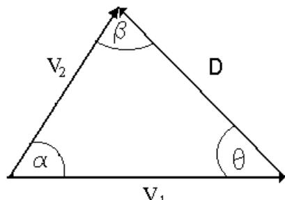
$$D = \sqrt{V_1^2 + V_2^2 - 2V_1V_2\cos\alpha}$$
